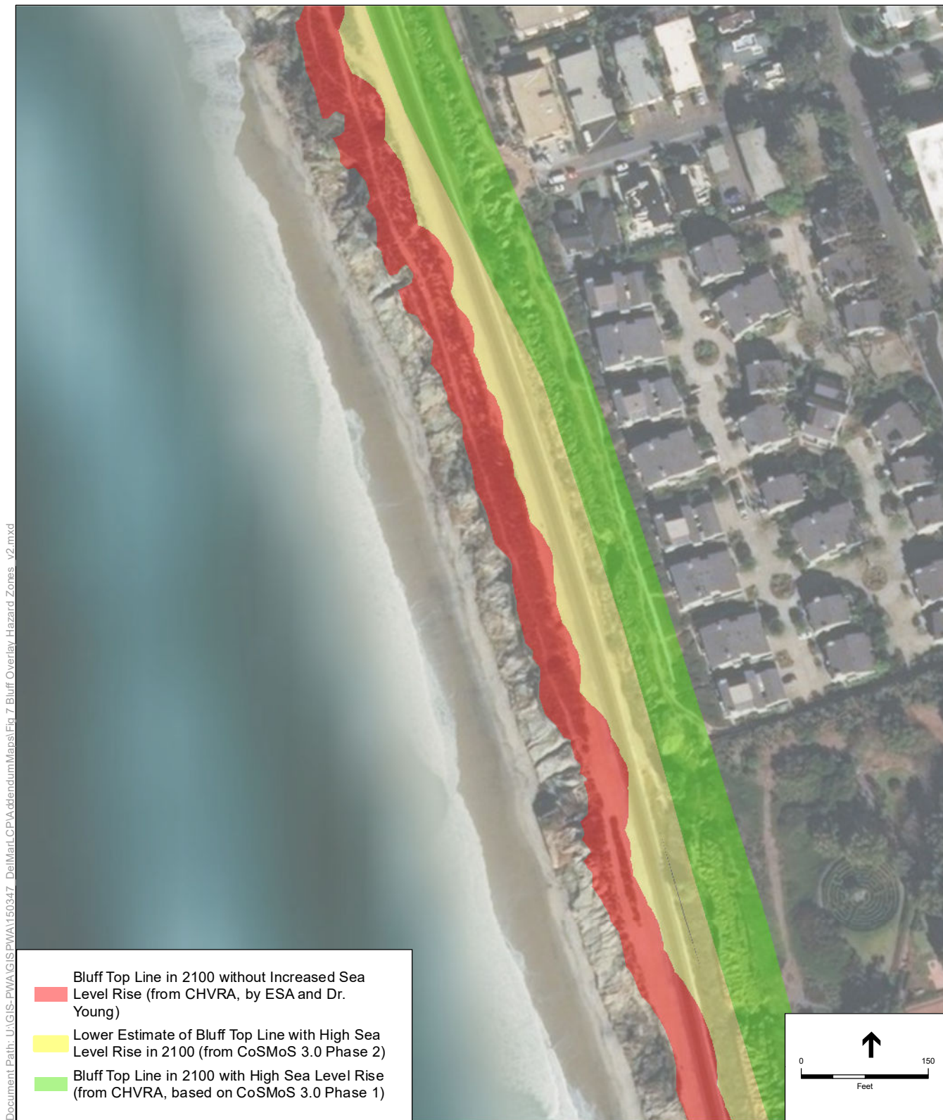
Del Mar Vulnerability Assessment Figure 7-6 Bluff Erosion Hazard Risk Zones
