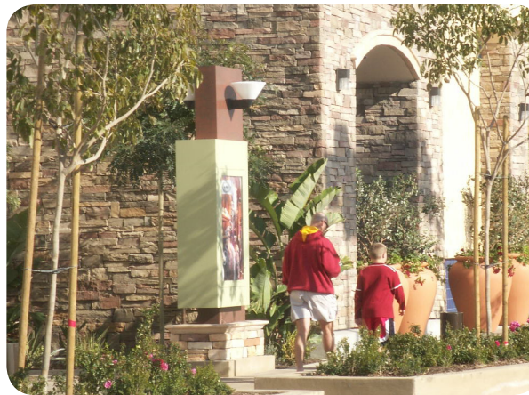
✗ Lighting should not direct light into the night sky.
