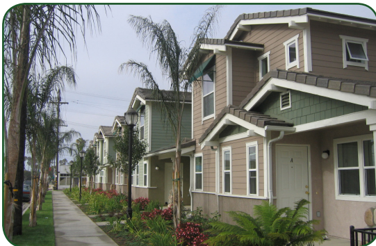
✓ Each dwelling unit has an individually recognizable entry, varied setbacks and roof planes and articulation.
