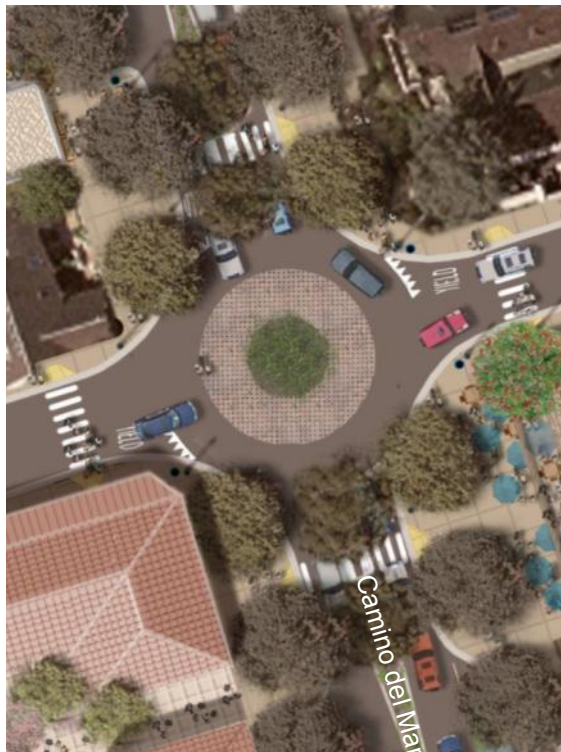
Roundabouts provide more traffic efficiencies than four-way stop signs and shorter distances for pedestrians to cross.
