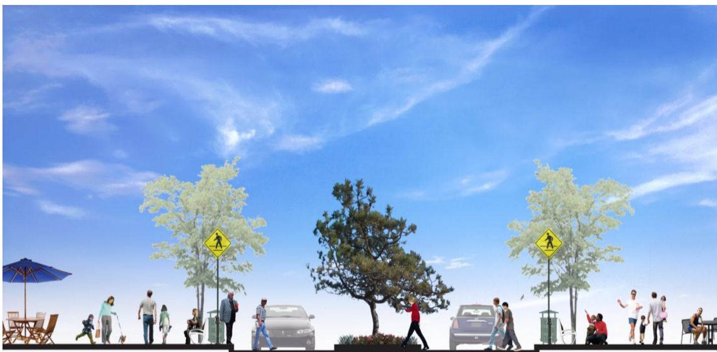
Figure IV-5, Crossing distance reduces from 80 feet to 34 feet: New plazas are provided at corners.
