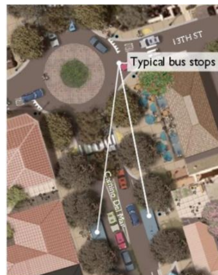
Bus stops would be in pullouts so as not to block traffic.
