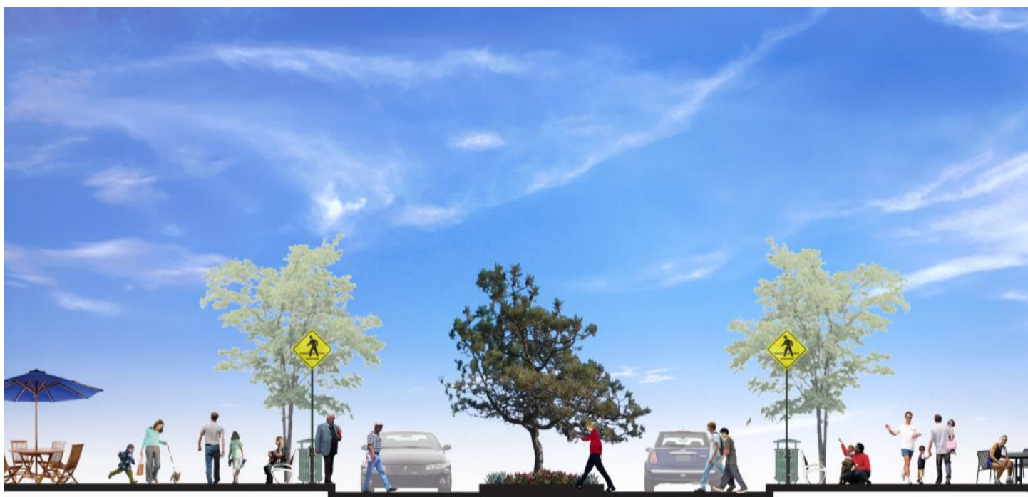
Figure IV-5, Crossing distance reduces from 80 feet to 24 feet: New plazas are provided at corners.
