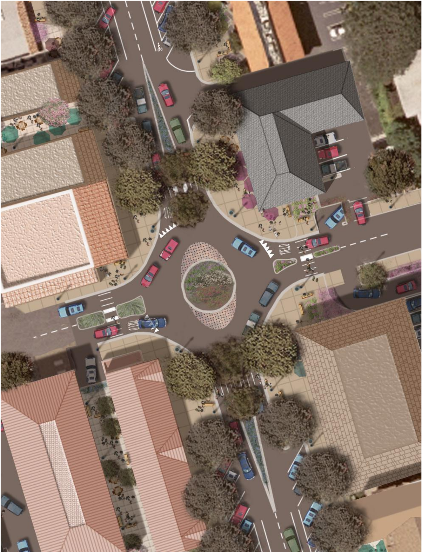
Figure IV-3, An illustration of proposed I Ith Street Roundabout and pedestrian improvements
