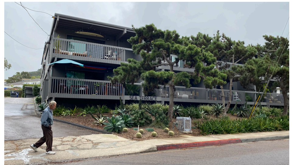
Limit the size of decks so they do not extend the full length of a facade, contributing to building bulk.
